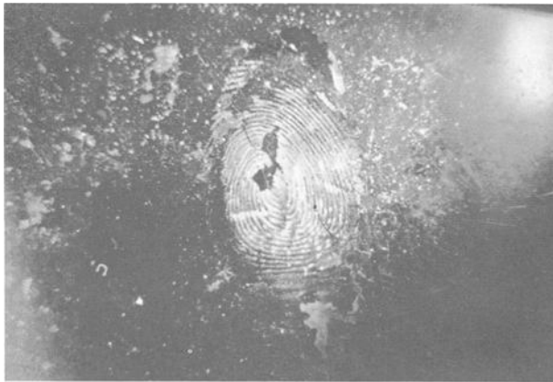
FIG. 4—The same bloody fingerprints as Fig. 1 viewed with the Nd: YAG laser.
